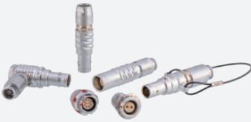
Push-pull connectors in the vibration sensor industry are mainly available in three series: 00, 0B and 1B. Mainly include 5pin, 6pin, 7pin and other pin numbers. Mainly used for acceleration vibration sensors, with fast plugging and unplugging characteristics, high efficiency. In addition to the push-pull type, there are also coaxial connectors. Temperature range: -25 to +75°C, high and low temperature products can be customized upon request.
