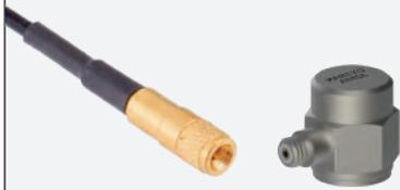
M3 series sensor plug, coaxial type connector. Product Thread Size: 5-44 UNF. Used for 1-axis acceleration sensor, and the matching connectors are BNC, SMB, L5 and other RF connectors. The ultra-low noise double-shielded coaxial cable used is specially treated to eliminate electrical noise.
