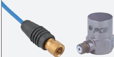
L5 series sensor plug, coaxial type connector. Product Thread Size: 10-32 UNF. Used for 1-axis acceleration sensor, and the matching connectors are BNC, SMB, M3 and other RF connectors. The ultra-low noise double-shielded coaxial cable used is specially treated to eliminate electrical noise.
