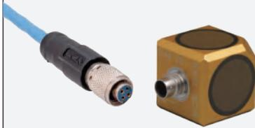
The C4 series connectors are the most popular small vibration sensor connectors on the market today, 4pin, Product Thread Size: 1/4 28 UNF. Used for 3-axis acceleration sensors, and its matching connectors are BNC, SMB and other RF connectors. Used low-noise cable, split three ways. Temperature range: -25 to +125°C, high and low temperature products can be customized upon request.
