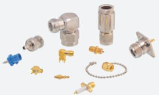
Coaxial connectors, in addition to the 3-56, 5-44, 10-32 sensor side connectors, will be used for BNC, SMB and other types of connectors, mainly used for acceleration and vibration sensors and ancillary testing equipment, ultra-low noise dual screen coaxial cable. Temperature range: -25 to +85°C, high and low temperature products can be customized upon request.
