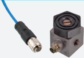
The C3 Series connectors are the smallest vibration sensor connectors on the market today, 4pin, Product Thread Size: 8-36 UNF. Used for 3-axis acceleration sensor, and its matching connectors are BNC, SMB and other RF connectors. Used low-noise cable, split three ways. Temperature range: -25 to +125°C, high and low temperature products can be customized upon request.
